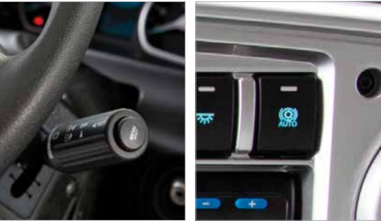
Engine brake and Intarder operating lever: You can manually activate the auxiliary brakes, or you can enable the vehicle to set it automatically for you.
