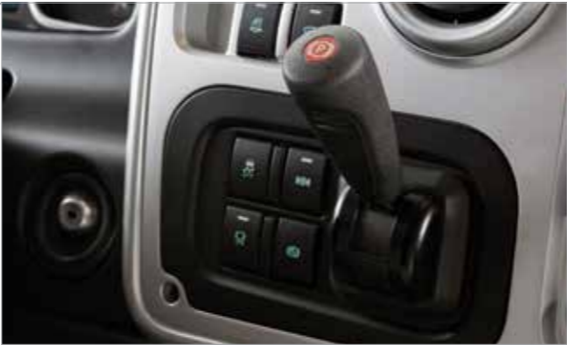
ESP, Hillholder and the trailer brake buttons are positioned to allow ease of access.
