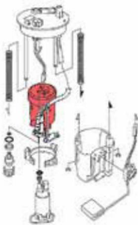
When refueling during ordinary use of the car, fine dirt may enter the fuel tank when opening and closing the fuel cap and this can build up within the fuel filter, and cause it to become blocked.
