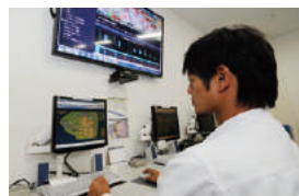
FEMS is used for centralized energy management of the entire plant (right: FEMS control screen)
