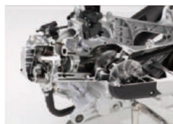
Global engine for next-generation compact scooters (cut-away model)
