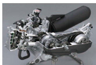
Newly developed eSP, a water-cooled, four-stroke overhead cam, single-cylinder 50-cc engine
