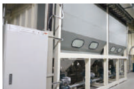
Dry spray booth installed for bumper coating
