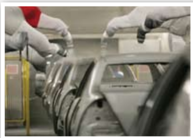
Water-based coatings, which contain fewer substances of concern, are used on painting lines at the Marysville automobile factory.
