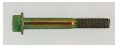
Traditional bolt containing hexavalent chromium
